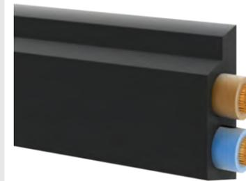
The flat cable is used for the voltage supply of ConveyorControl and MultiControl. The outer contour of the line corresponds to the standard of AS interface. The shell of the line covers holes that were created by penetration contacts. This means that the cable maintains the protection rating even after disconnecting a control.
