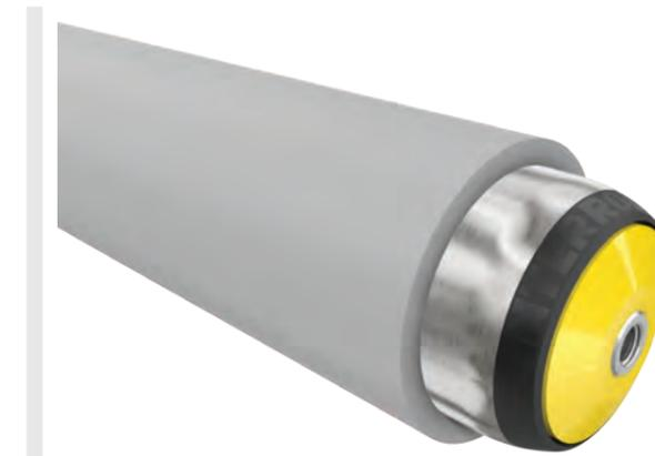
The PVC sleeve ensures a particularly high noise reduction and offers a high level of protection for sensitive materials. An improved conveyance of materials is achieved with the higher coefficient of friction compared with a steel tube. Materials can easily be separated since the larger diameter leads to a higher speed with the same rotational speed.
