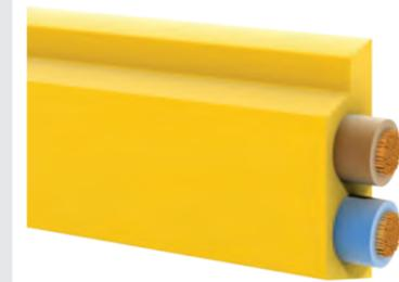
The flat cable is used for the communication of the ConveyorControl control system. The different controls of the system simply contact the line via penetration contacts. The outer contour of the line corresponds to the standard of AS interface. The shell of the line covers holes that were created by penetration contacts. This means that the cable maintains the protection rating even after disconnecting a control.
