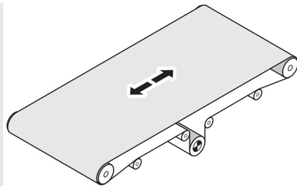
Fig.: Long belt conveyor with center drive
