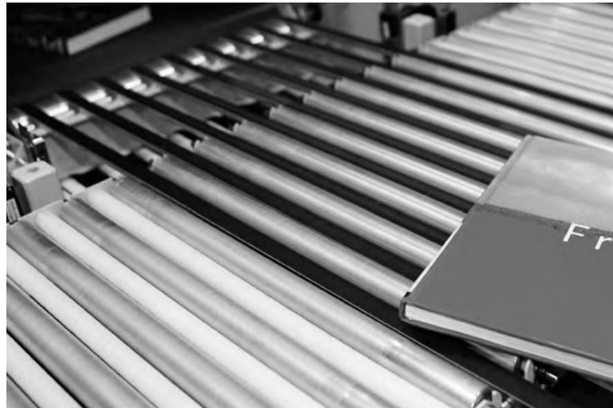
All Interroll Drum Motors excel with relatively low noise development and vibrations. The performance levels are not specified or guaranteed in this catalog because they can vary depending on the type of motor, number of poles, speed and application. For specific low-noise applications, please contact your Interroll customer consultant.
