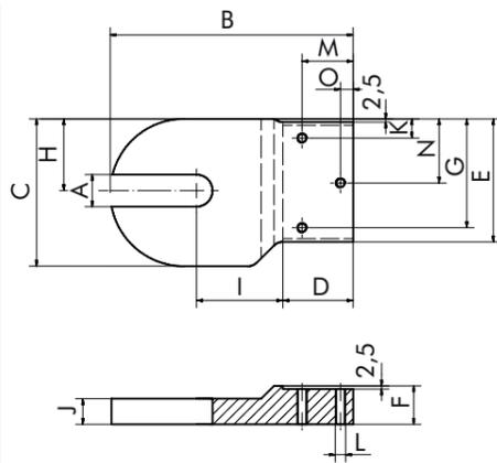
Fig.: Right bracket (A) aluminum or VA
