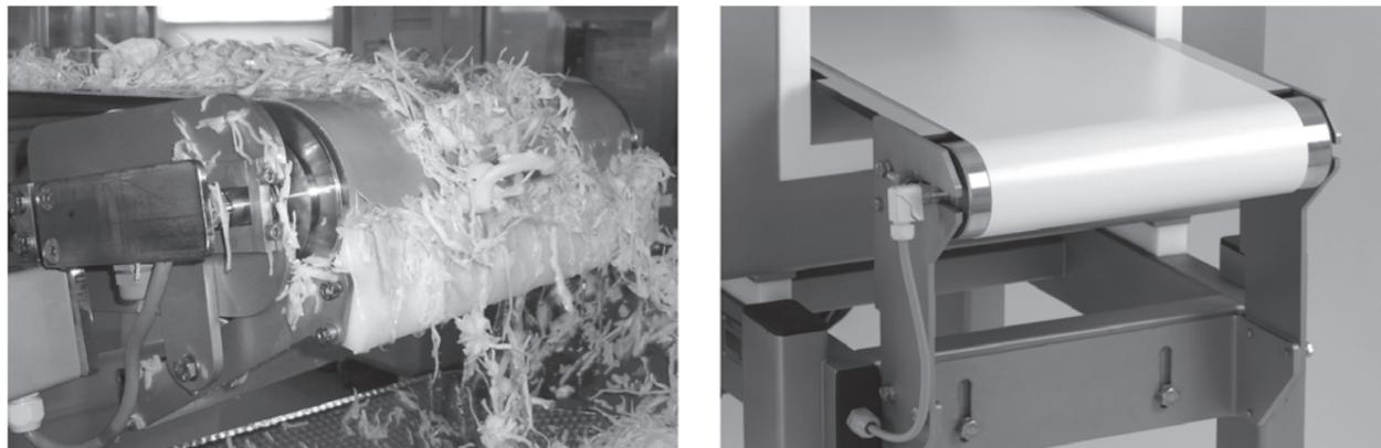
Friction drive belts are driven via the friction between drum motor and conveyor belt. The drum motor is normally crowned to prevent belt wander. The belt must be tensioned in order to transfer the torque from the drum motor. The top surface of the belt can be flat, plain or have a ribbed, grooved or diamond pattern.
