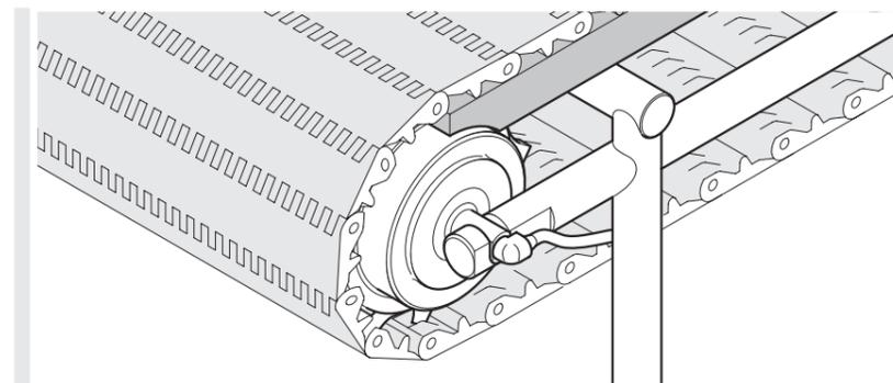
Fig.: Open conveyor design for hygienic cleaning
