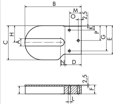
Fig.: Right bracket (C) aluminum or PE
