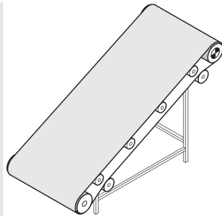
Fig.: Inclined conveyor
