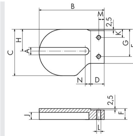
Fig.: Right bracket (C) aluminum or VA
