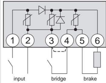
Fig.: Half-wave rectifier
