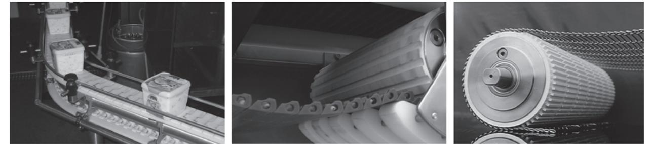
Modular plastic belts, solid homogeneous belts, steel mesh or wire belts are positively driven, i.e., with no belt tension. Since the belt has hardly any direct contact with the drum shell, the heat dissipation is less effective in these applications. For this reason, the drum motor should be used with a frequency inverter that is optimized for this application.
