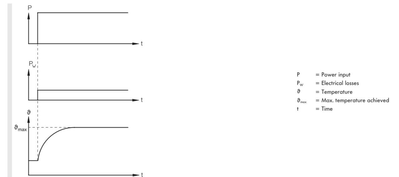
The majority of Interroll Drum Motor windings with an efficiency of over 50 % are suitable for operating mode S1 and continuous running duty. Please refer to the electrical data tables for standard motors and motors for applications with positive drive belts or no belts. The value is listed with the symbol  $\eta$  for efficiency.
