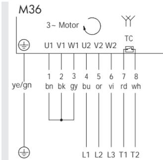
Fig.: 3-phase, 7+2 core cable, 2 speeds, double-star connection
