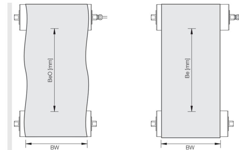
Fig.: Measuring the belt elongation
