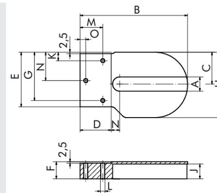
Fig.: Left bracket (B) aluminum or PE
