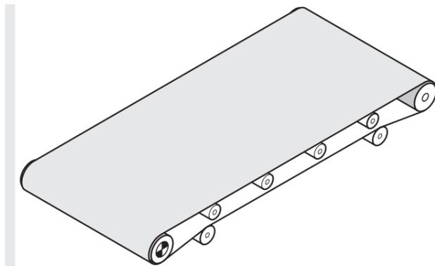
Fig.: Roller bed conveyor
