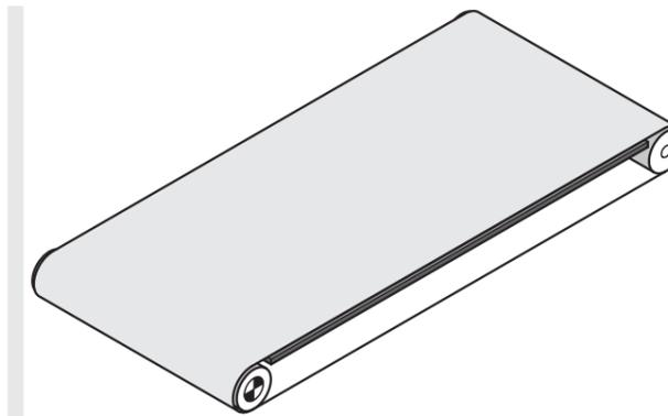
Fig.: Slider bed conveyor
