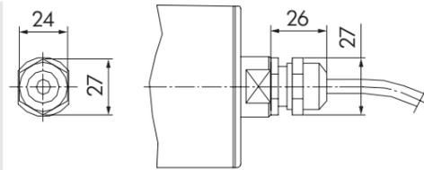
Fig.: Straight connector, brass or stainless steel
