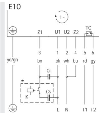
Fig.: 1-phase, 7-core cable
