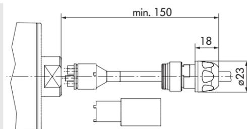
Fig.: Mounting dimensions with a mounting tool
