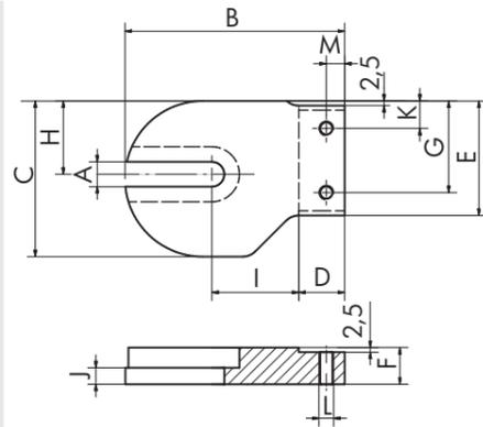
Fig.: Right bracket (A) aluminum or VA
