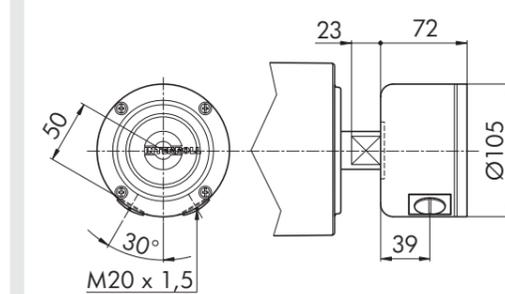
Fig.: DM 0113, terminal box, technopolymer
