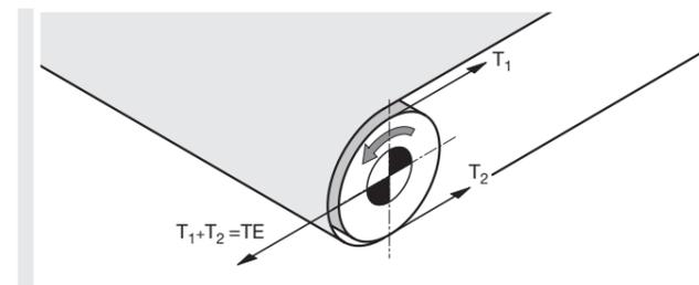
The required belt tension T1 (top side) and T2 (bottom side) can be calculated in accordance with DIN 22101 or the CEMA standard. Based on the information from the belt manufacturer, the actual belt tension can be roughly determined by a measurement of the belt elongation during tensioning.
