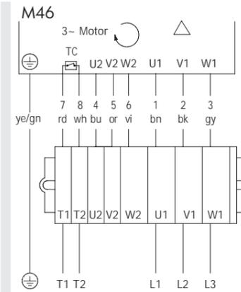
Fig.: 3-phase, 7+2 core cable, 2 speeds, delta connection
